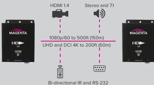
The HD-One DX series is available in HDBaseT and extended range variants in a compact form factor for the transmission of HDMI 1.4 signals including 1080p, 3D, UHD/4K and 4K DCI. Together, the HD-One DX series has full audio support including LPCM 7.1CH, Dolby, TrueHD, Dolby Digital Plus and DTS-HD.
