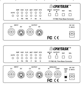
Connect the AC to +12 VDC adapter to an AC source and then to the DC power input shown above. (Note that there is no power switch. The unit will begin to work as soon as you have the AC to +12 VDC adapter plugged in and furnishing power).
