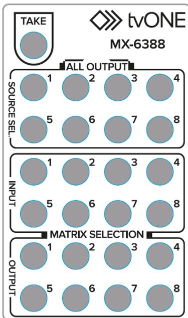
Normal matrix functions are performed by pressing the numbered button of the input you wish to route from the two rows of “INPUT” buttons followed by pressing the numbered button(s) of the desired output(s) from the two rows of “OUTPUT” buttons.
